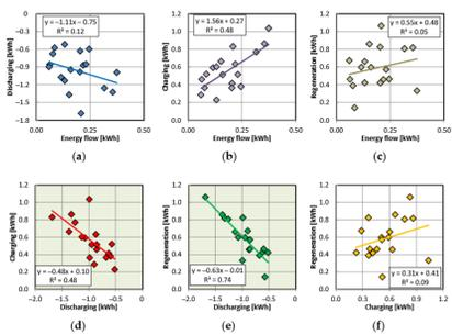
Comparative analysis of the relation: (a-c) between total energy flow, discharge energy, charging energy and energy recovered during vehicle braking; (d-f) between energy recovered during vehicle braking, charging and discharging. Pielecha, I.; Cieslik, W.; Szwajca, F. (2023)
